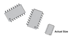
Vishay Dale Thin Film offers standard circuits in 16 pins in a medium body molded surface mount package. The networks are available over a resistance range of 100  $\Omega$  to 100  $k\Omega.$  The network features tight ratio tolerances and close TCR tracking. In addition to the standards shown, custom circuits are available upon request.
