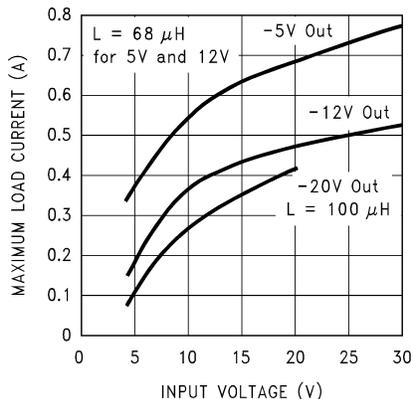
Figure 22. Maximum Load Current for Inverting Regulator Circuit
