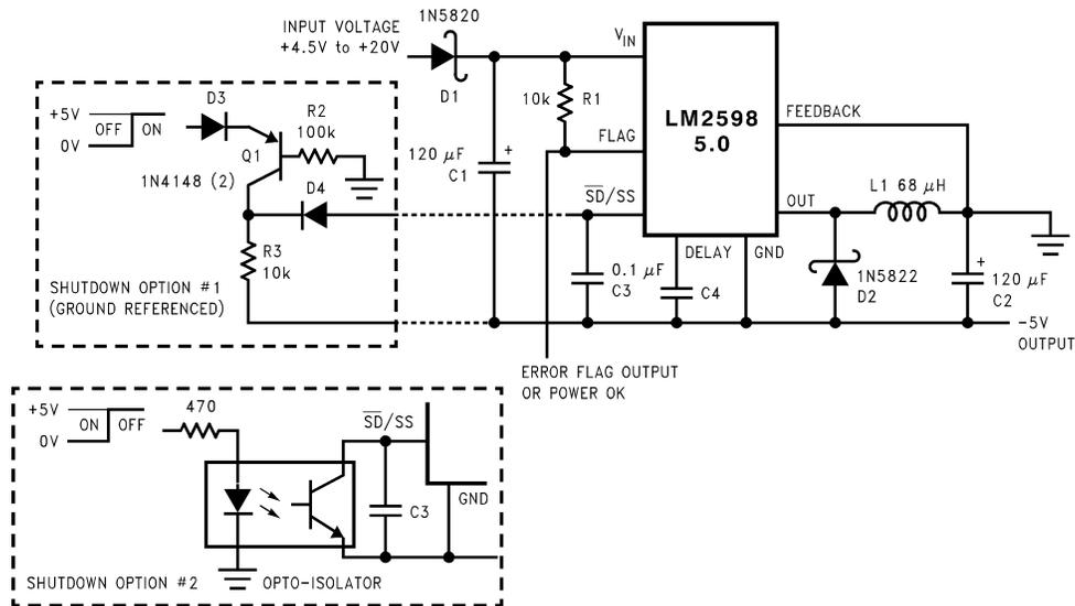
Figure 21. Inverting -5-V Regulator With Shutdown and Soft-start
