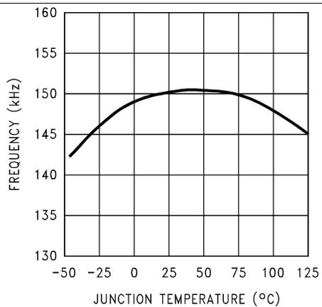
Figure 12. Switching Frequency
