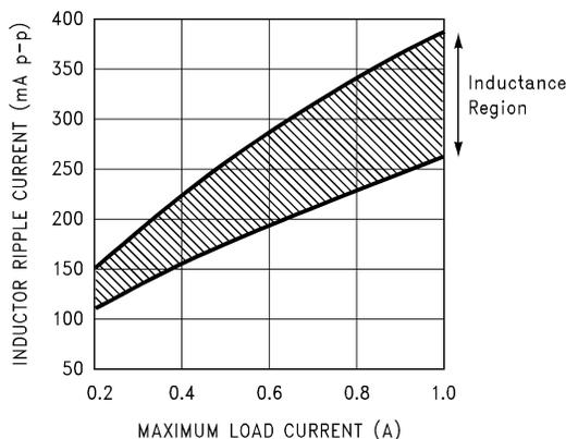
**Figure 39. Peak-to-Peak Inductor Ripple Current vs Load Current**
