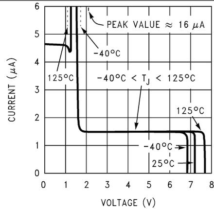
Figure 14. Shutdown/Soft-start Current
