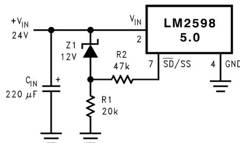
**Figure 23. Undervoltage Lockout for a Buck Regulator**
