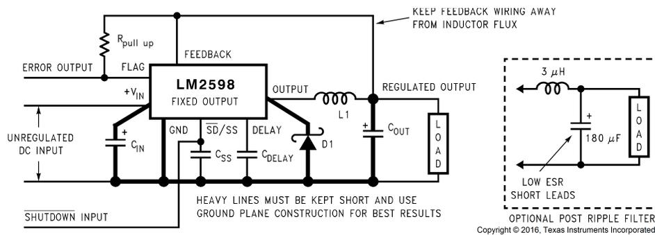
Component Values shown are for  $V_{IN} = 15\text{ V}$ ,  $V_{OUT} = 5\text{ V}$ ,  $I_{LOAD} = 1\text{ A}$ .
