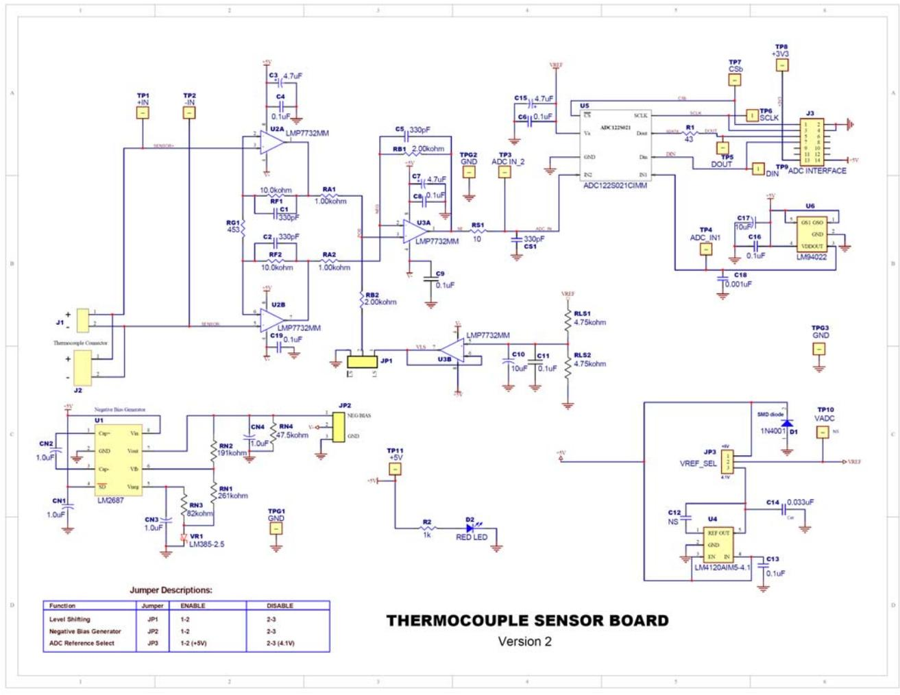
Figure 2. Thermocouple Sensor Board Version 2 Schematic
