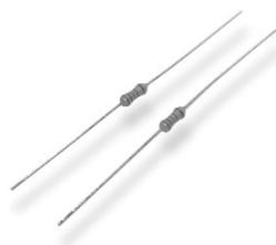
The resistive element comprises a thin film of nickel-chrome alloy evaporated onto a high thermal conductivity ceramic element. Metal end caps are force fitted to the element prior to spiralling to value. Tinned copper lead wires are welded to the end caps and the components are then coated. One coat of phenolic resin is followed by three coats of epoxy resin. All resistors are tested for value and tolerance.
