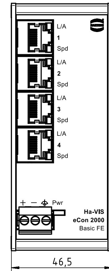
for mounting rail acc. to DIN EN 60715
