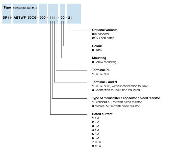
The rated current of the line-filter must not be exceeded in the end application.
