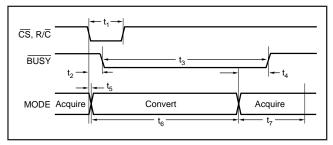
FIGURE 1. Basic Conversion Timing.
