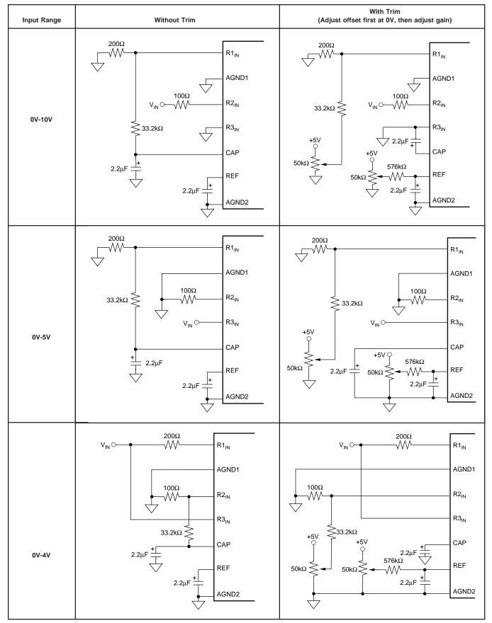
FIGURE 4a. Offset/Gain Circuits for Unipolar Input Ranges.
