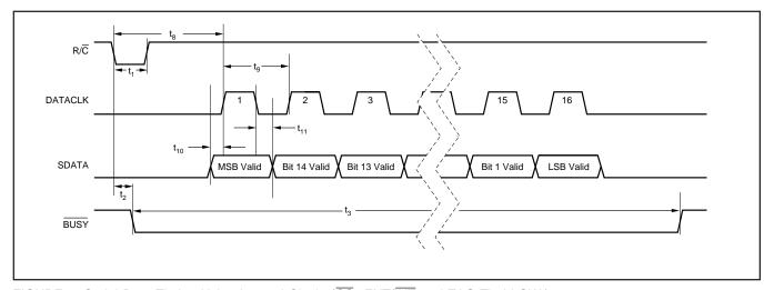
FIGURE 2. Serial Data Timing Using Internal Clock. ( $\overline{\text{CS}}$ , EXT/ $\overline{\text{INT}}$  and TAG Tied LOW.)
