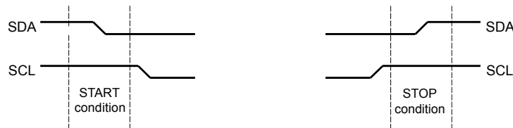
Figure 16-3. START and STOP Conditions
