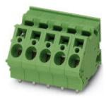
PCB terminal block, nominal current: 32 A, nom. voltage: 630 V, pitch: 7.5 mm, number of positions: 4, connection method: Spring-cage connection, mounting: Wave soldering, conductor/PCB connection direction: 45 °, color: multi-color
