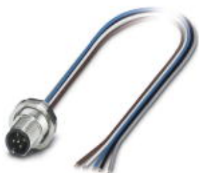
Sensor/actuator flush-type plug, 5-pos., M12, A-coded, rear/screw mounting with Pg9 thread, with 1.5 m TPE litz wire, 5 x 0.34 mm²
