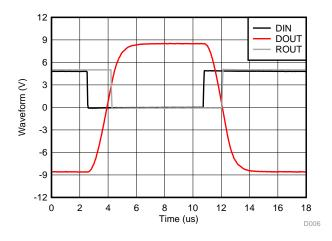
120 kbit/s, 1-nF load Figure 13. Driver and Receiver Loopback Signal
