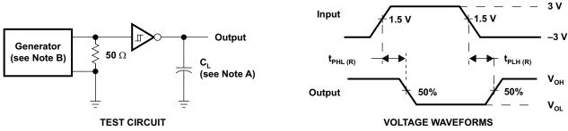
A. C<sub>L</sub> includes probe and jig capacitance.
