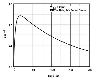
Figure 12. Typical HBM Current Waveform
