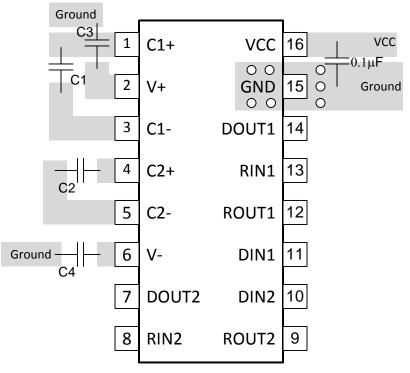
Figure 14. MAX202 Circuit Board Layout
