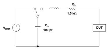
Figure 11. HBM ESD Test Circuit
