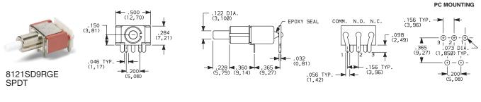
Not available with JXX actuators, D3, H, H9, Y3, Y4 bushings, I seal option. R termination not UL/CSA approved.
