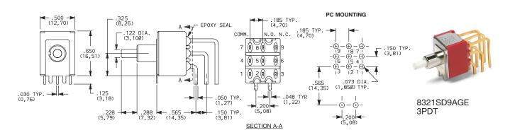
Not available with JXX actuators and I seal option. Terminal bend radii and lead-in manufacturing option
