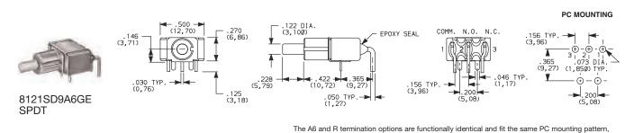
Not available with JXX actuators, D3, H, H9, Y3, Y4 bushings and I seal. Terminal bend radii and lead-in manufacturing option.
