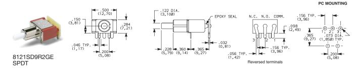
Not available with JXX actuators, D3, H, H9, Y3, Y4 bushings, I seal option. R2 termination not UL/CSA approved.
