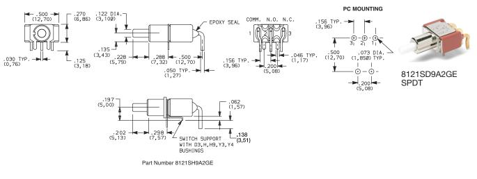
Not available with JXX actuators, I seal option. Terminal bend radii and lead-in manufacturing option.
