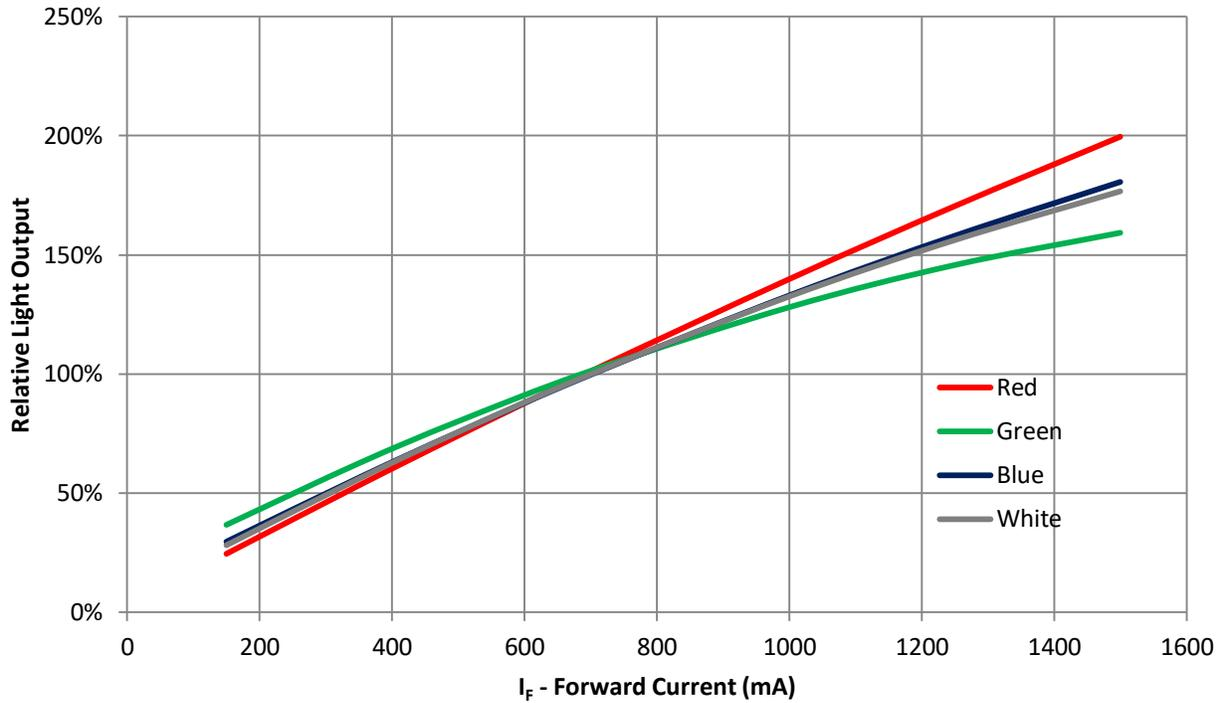
Figure 7: Typical relative light output vs. forward current @ T<sub>c</sub> = 25°C
