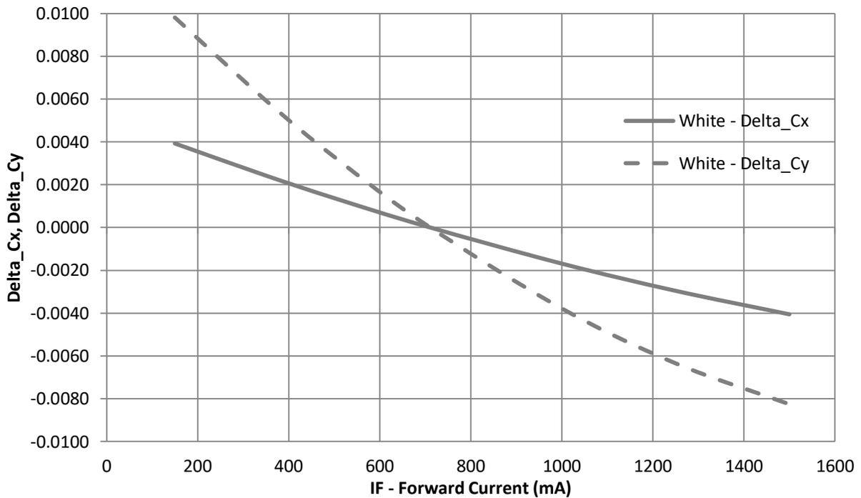
Figure 9b: Typical chromaticity coordinate shift vs. forward current @ T<sub>C</sub> = 25°C.
