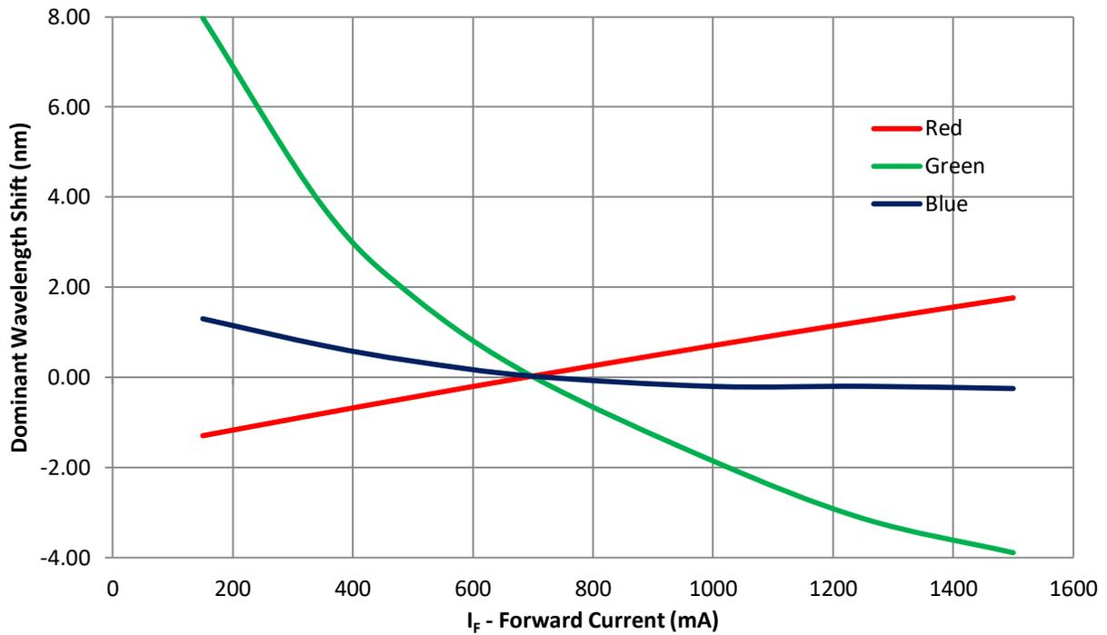
Figure 9a: Typical dominant wavelength shift vs. forward current @ T<sub>C</sub> = 25°C.
