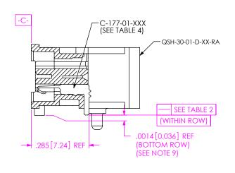
IN-PROCESS 1 (FILL BOTTOM ROW) (SEE INSPECTION VIEW 1 FOR ORIENTATION AND CPC'S)
