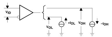
Figure 6. Receiver,  $V_{\text{OH}}$  and  $V_{\text{OL}}$
