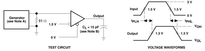
Figure 7. Receiver Propagation-Delay Times
