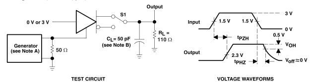
Figure 4. Driver Enable and Disable Times
