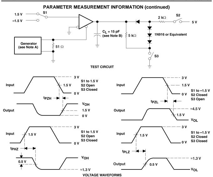
Figure 8. Receiver Output Enable and Disable Times
