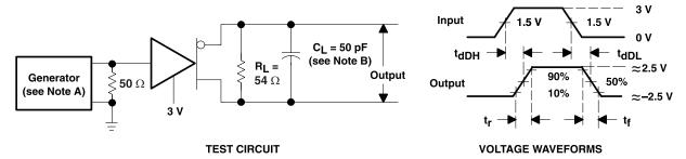
Figure 3. Driver Differential-Output Delay and Transition Times
