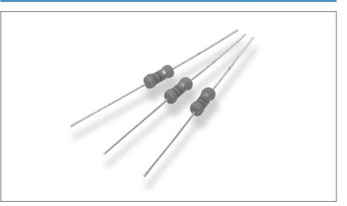
The resistive element comprises a metal oxide film deposited on a ceramic former. The element is protected by a flameproof coating which will withstand overload conditions without flame or mechanical damage. They are recommended for use in applications such as line protection etc...
