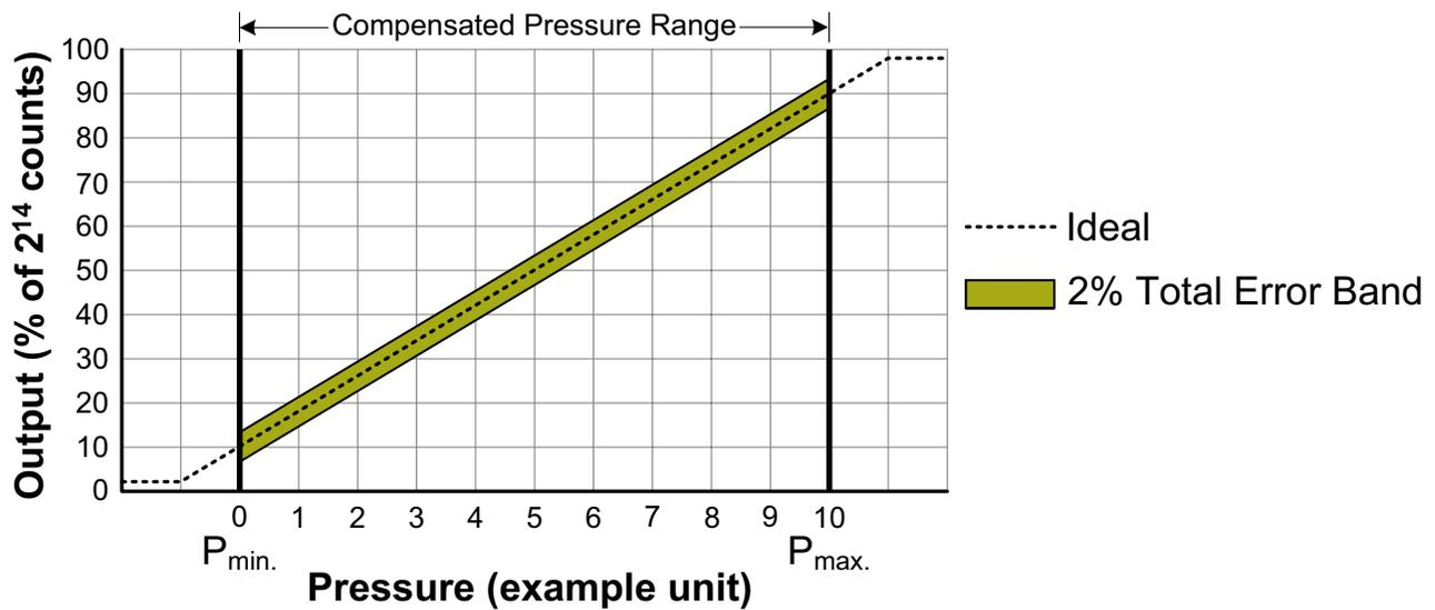
$$\text{Output (\% of } 2^{14} \text{ counts)} = \frac{80\%}{P_{\text{max.}} - P_{\text{min.}}} \times (\text{Pressure}_{\text{applied}} - P_{\text{min.}}) + 10\%$$
