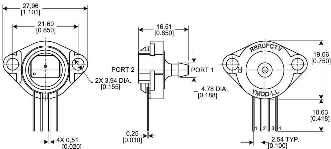
**SIP NB:** Fastener mount, dual axial ports, same side
