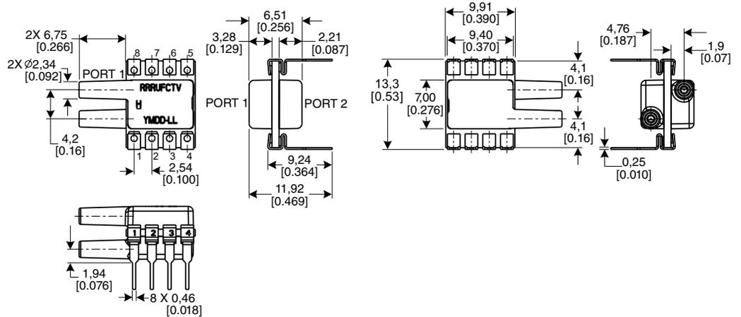
Figure 7. SMT Package Dimensional Drawings (For reference only: mm [in].)
