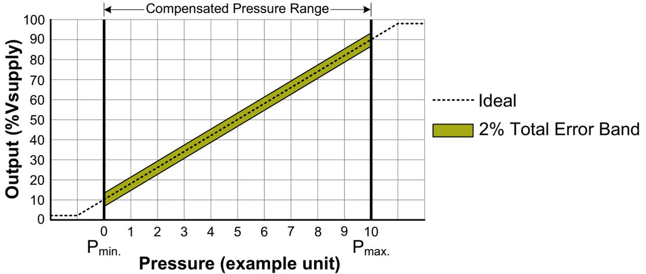
$$\text{Output (V)} = \frac{0.8 \times V_{\text{supply}}}{P_{\text{max.}} - P_{\text{min.}}} \times (\text{Pressure}_{\text{applied}} - P_{\text{min.}}) + 0.10 \times V_{\text{supply}}$$
