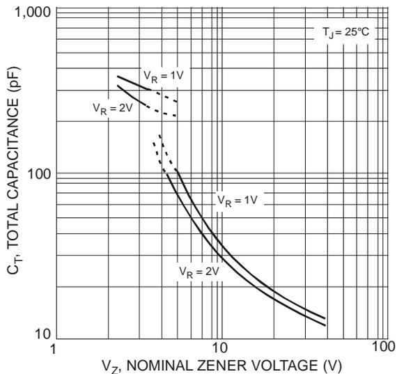
Fig. 5 Typical Total Capacitance vs. Nominal Zener Voltage
