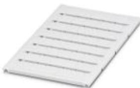
Marker for terminal blocks, Sheet, white, unlabeled, can be labeled with: BLUEMARK CLED, BLUEMARK LED, Plotter, Mounting type: Snap into tall marker groove, for terminal block width: 12 mm, Lettering field: 11.45 x 10.5 mm
