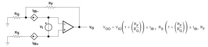
Figure 25. Output Offset Voltage Model
