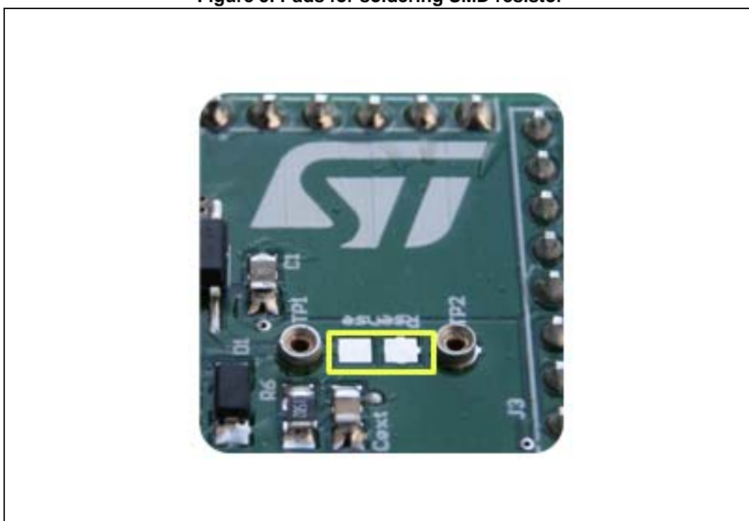
Figure 5. Pads for soldering SMD resistor
