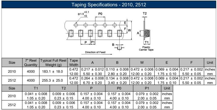
Note: Plastic carrier tape used for 2010 and 2512 sizes.
