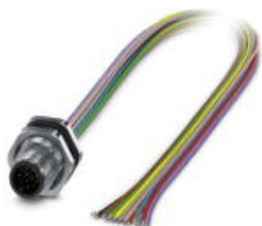
Flush-type connector, Universal, 8-position, Plug, M12, A-coded, Rear mounting, M16 x 1.5, Individual wires, cable length: 0.5 m
