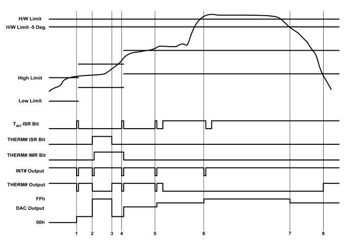
Figure 14. LM87 Interrupt Structure
