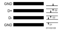
Figure 12. Recommended Diode Trace Layout
