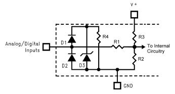
Figure 2. ESD Protection Input Structure
