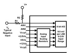
Resistor values shown in Table 2 provide approximately 1.25V at the Vccp inputs.
