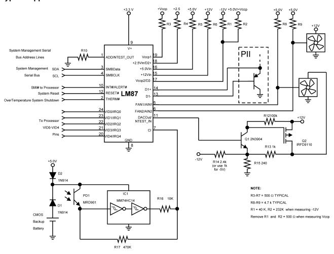
In this PC application the LM87 monitors temperature, fan speed for 2 fans, and 6 power supply voltages. It also monitors an optical chassis intrusion detector. The LM87 provides a DAC output that can be used to control fan speed.
