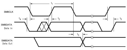
Figure 1. Serial Bus Timing Diagram
