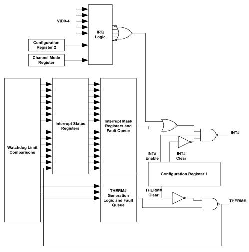
Figure 13. Interrupt Structure
