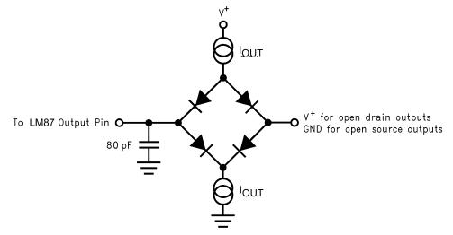
Figure 3. Digital Output Load Test Circuitry
