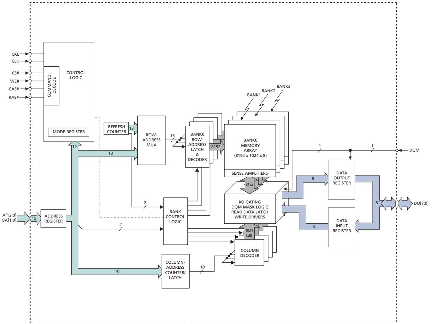
Figure 3: 16 Meg x 16 Functional Block Diagram
