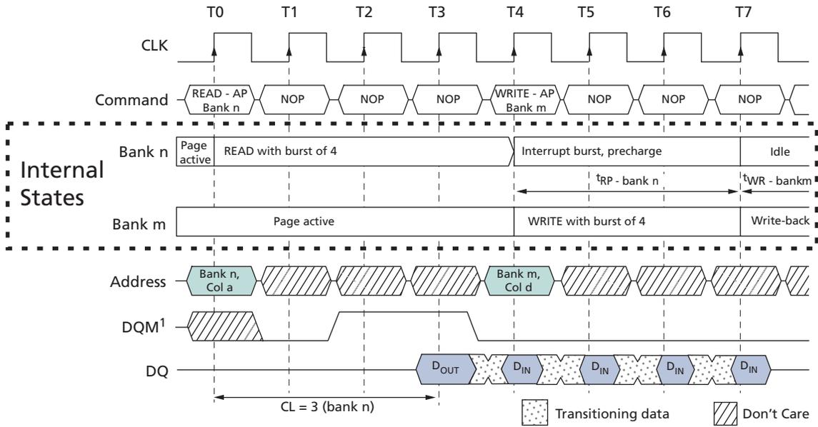
Note: 1. DQM is HIGH at T2 to prevent D<sub>OUT</sub> a + 1 from contending with D<sub>IN</sub> d at T4.
