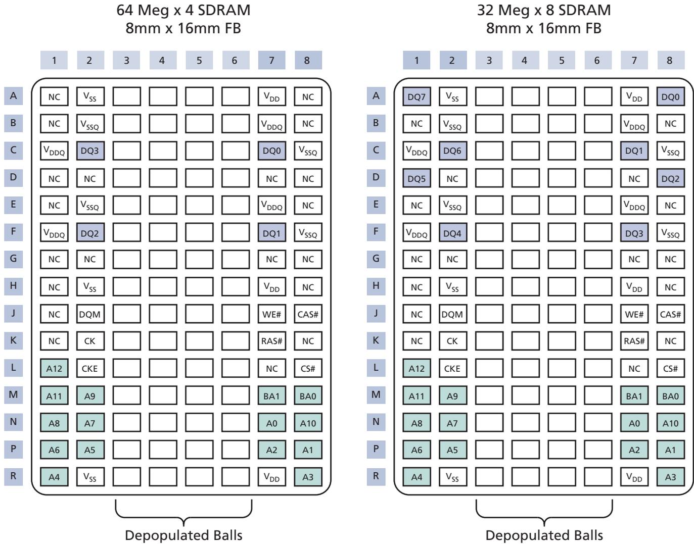
**Figure 6: 54-Ball VFBGA (Top View)**
