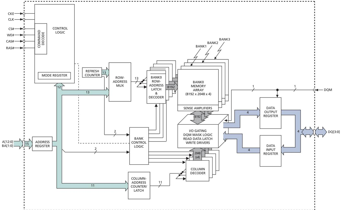
Figure 2: 32 Meg x 8 Functional Block Diagram
