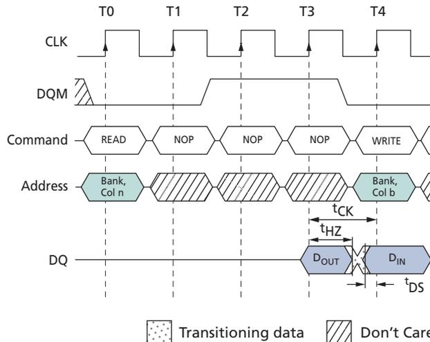
Note: 1. CL = 3. The READ command can be issued to any bank, and the WRITE command can be to any bank. If a burst of one is used, DQM is not required.
