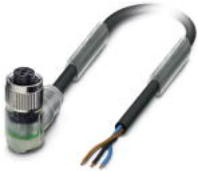
Sensor/actuator cable, 3-position, PUR halogen-free, black-gray RAL 7021, free cable end, on Socket angled M12, coding: A, with 2 LEDs, cable length: 5 m
