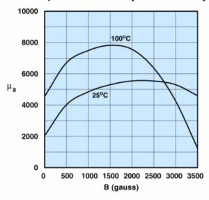
Measured on an 18/10/6mm toroid at 10kHz.
