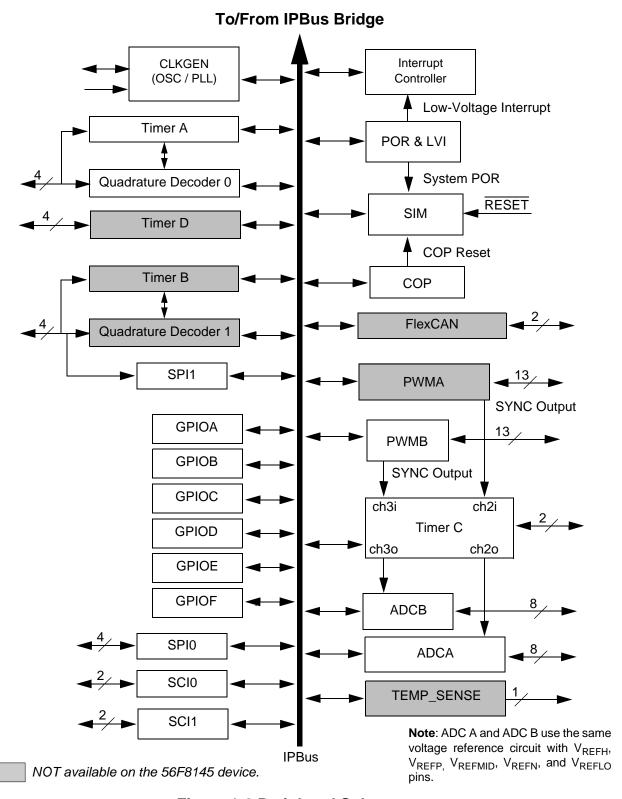
Figure 1-2 Peripheral Subsystem
