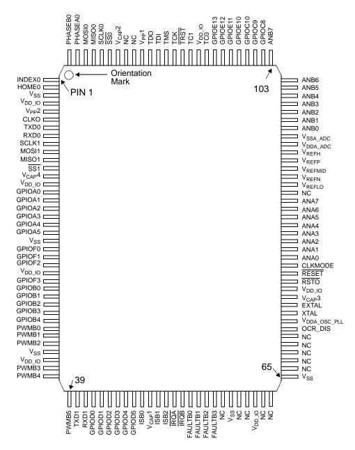
Figure 11-2 Top View, 56F8145 128-pin LQFP Package
