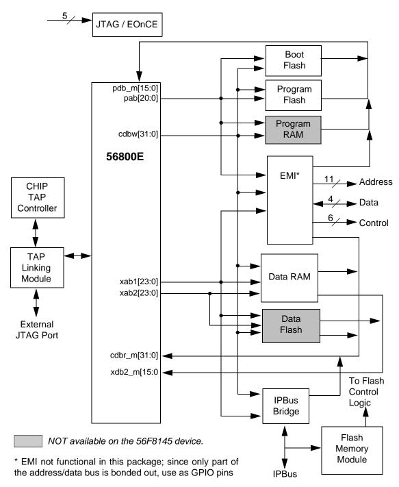
Figure 1-1 System Bus Interfaces
