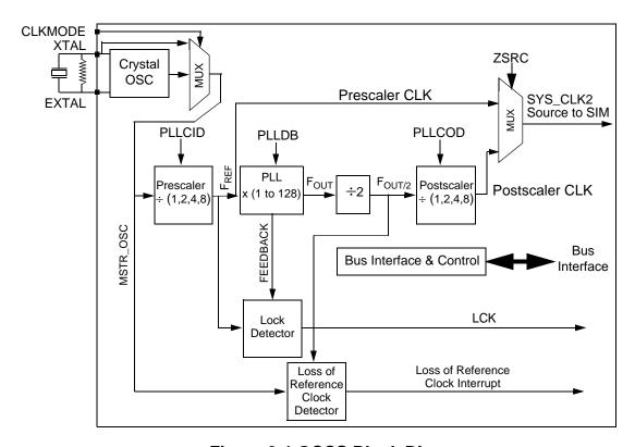
Figure 3-1 OCCS Block Diagram
