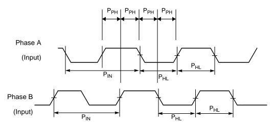
Figure 10-14 Quadrature Decoder Timing
