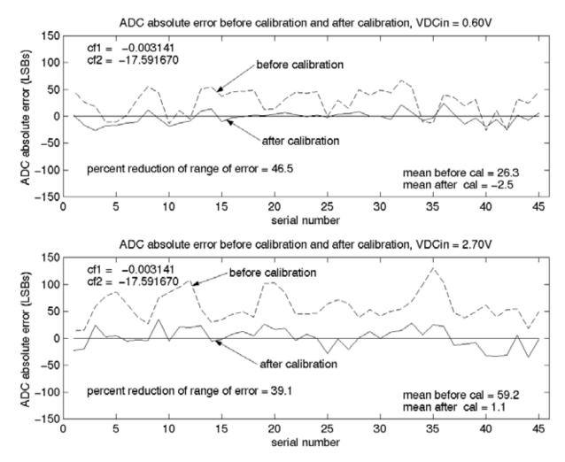
Figure 10-21 ADC Absolute Error Over Processing and Temperature Extremes Before and After Calibration for VDC<sub>in</sub> = 0.60V and 2.70V
