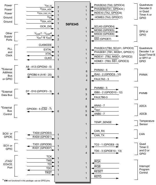
Figure 2-1 56F8345 Signals Identified by Functional Group<sup>1</sup> (128-Pin LQFP)
