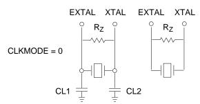
Sample External Crystal Parameters:  $R_z = 750 \text{ K}\Omega$
