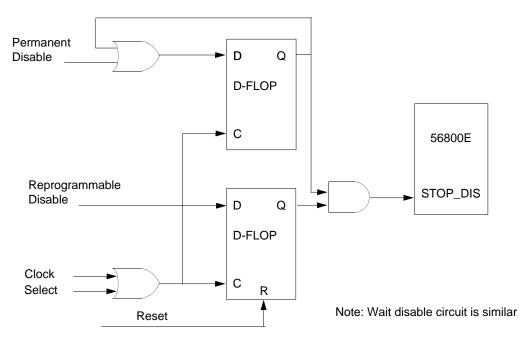
Figure 6-16 Internal Stop Disable Circuit
