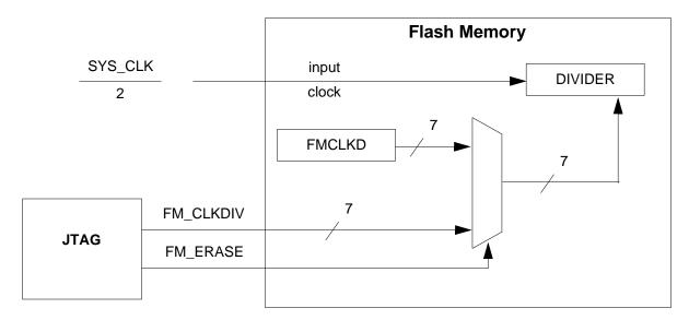
Figure 7-1 JTAG to FM Connection for Lockout Recovery
