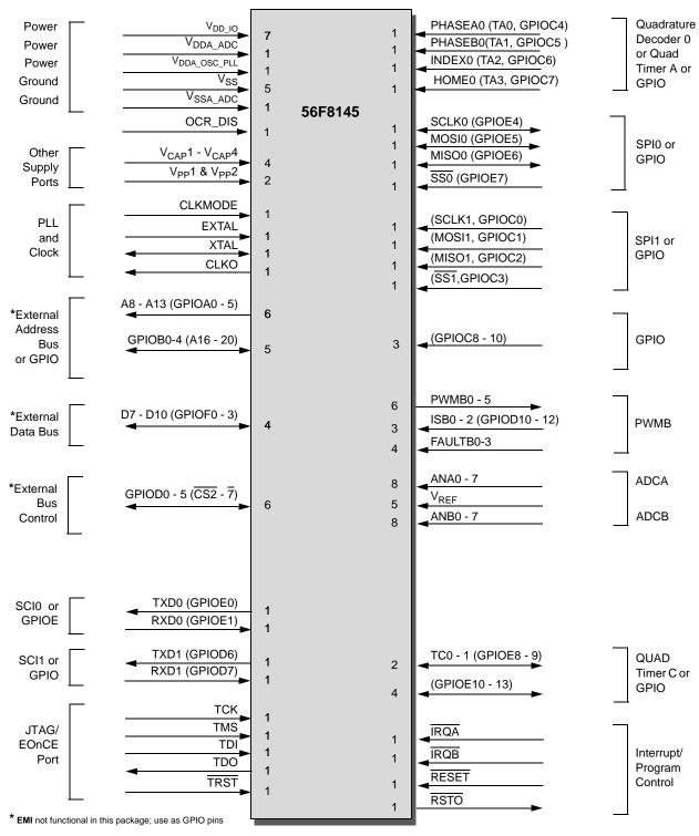
Figure 2-2 56F8145 Signals Identified by Functional Group<sup>1</sup> (128-Pin LQFP)
