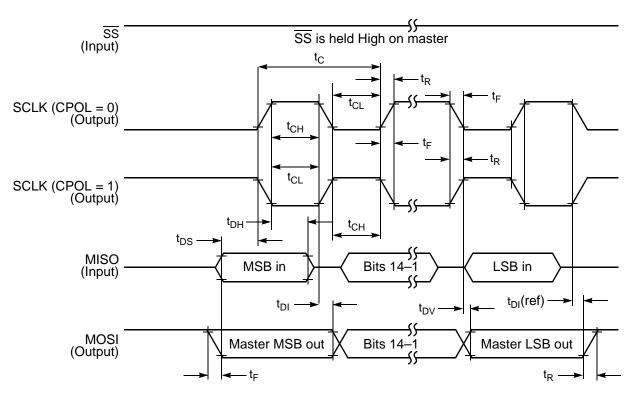
Figure 10-9 SPI Master Timing (CPHA = 0)
