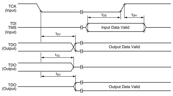
Figure 10-19 Test Access Port Timing Diagram
