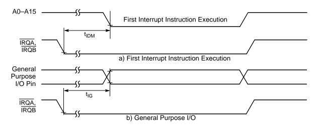
Figure 10-6 External Level-Sensitive Interrupt Timing
