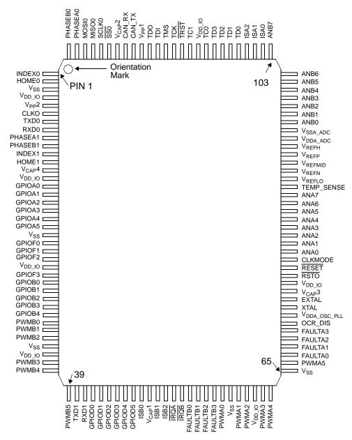
Figure 11-1 Top View, 56F8345 128-pin LQFP Package
