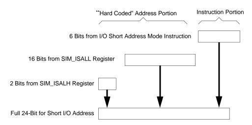
Figure 6-13 I/O Short Address Determination
