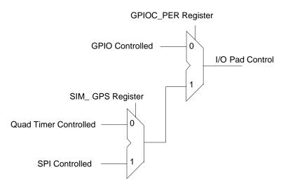
Figure 6-10 Overall Control of Pads Using SIM\_GPS Control
