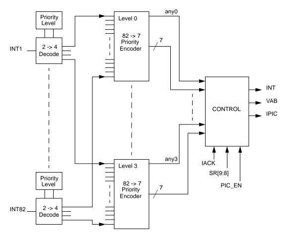
Figure 5-1 Interrupt Controller Block Diagram
