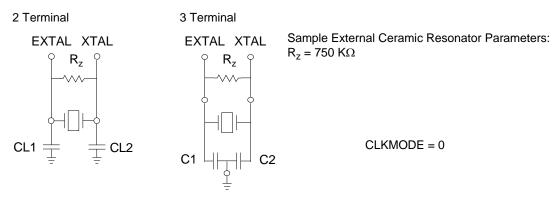
Figure 3-3 Connecting a Ceramic Resonator
