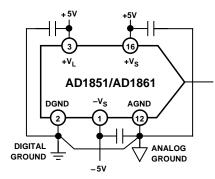
Figure 2. Recommended Circuit Schematic
