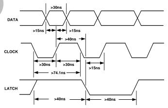
Figure 8. Timing Relationships of AD1861 Input Signals
