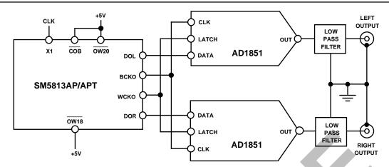
Figure 11. AD1851 with NPC SM5813AP/APT Digital Filter
