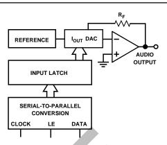
Figure 1. AD1851/AD1861 Functional Block Diagram
