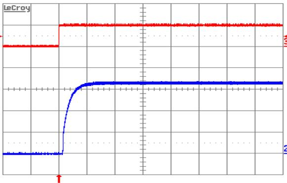
Figure 7: Turn-on transient at full rated load current (resistive) plus 20,000  $\mu\text{F}$  at  $V_{in} = 48\text{ V}$ , triggered via ON/OFF pin. Top trace: ON/OFF signal (5 V/div.). Bottom trace: Output voltage (1 V/div.). Time scale: 5 mS/div.
