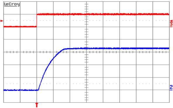
Figure 8: Output voltage response to load current step-change (10A–15A–10A) at  $V_{in}=48\text{V}$ . Top trace: output voltage (100 mV/div.). Bottom trace: load current (5A/div.). Current slew rate: 0.1A/ $\mu\text{s}$ .  $C_o=1\mu\text{F}$  ceramic + 10 $\mu\text{F}$  tantalum. Time scale: 0.2mS/div.
