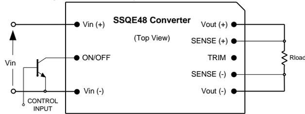
The positive logic version turns on when the ON/OFF pin is at a logic high and turns off when the pin is at a logic low. The converter is on when the ON/OFF pin is left open. See the Electrical Specifications for logic high/low definitions.
