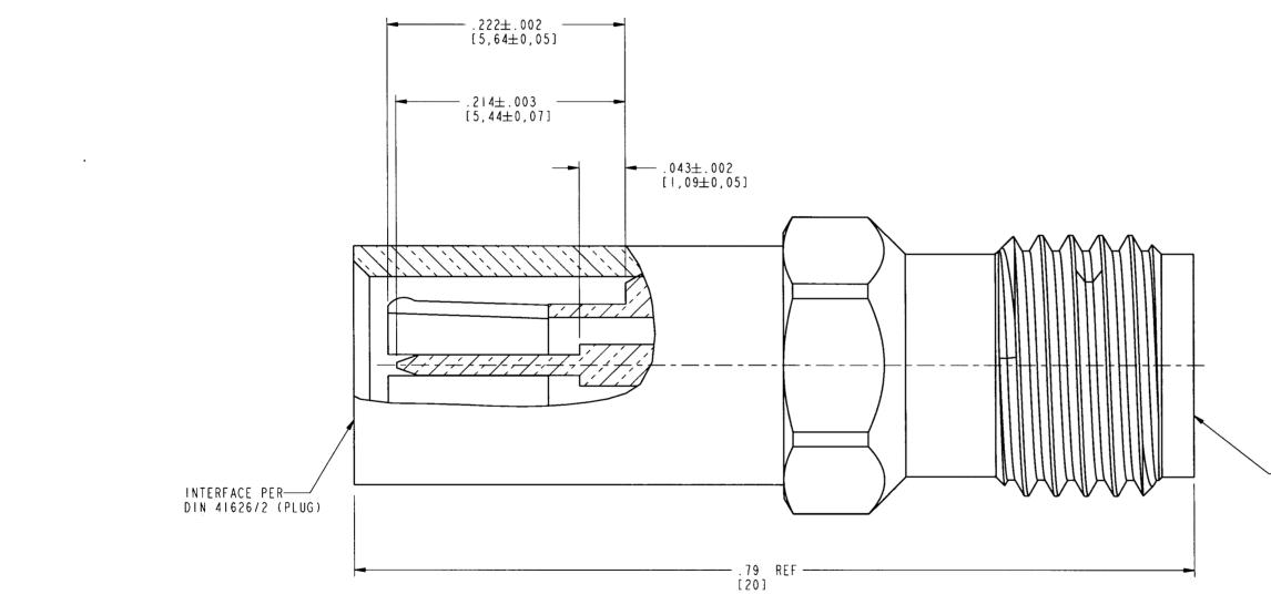
NOTES: I. MATERIAL AND FINISH: BODY - BeCu, GOLD PLATED CONTACT - BeCu, GOLD PLATED INSULATOR - PTFE 2. ELECTRICAL A. VSWR(RETURN LOSS), MAXIMUM DC - 4GHz: 1.15 (-30 dB)
