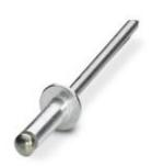
Blind rivets, Ø 4.0 mm, 6 mm sleeve length, aluminum sleeve, zinc-plated steel pin, flat head, standard version similar to DIN 7337 A
