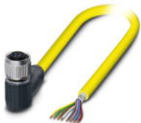
Sensor/actuator cable, 8-position, PVC, yellow, shielded, free cable end, on Socket angled M12 SPEEDCON, A-coded, cable length: 10 m
