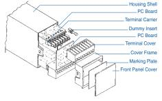
Fast On tab and the printed circuit board(s). Solder Tab can be hand soldered to the board.
