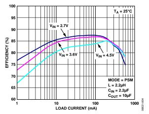
Figure 4. Efficiency vs. Load Current ( $V_{OUT} = 1.2 V$ )
