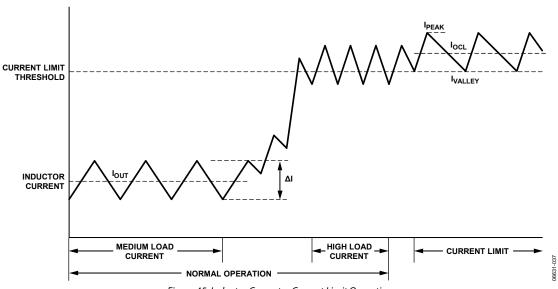
Figure 45. Inductor Current—Current Limit Operation
