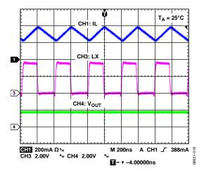
Figure 29. CCM Mode Operation at Medium/Heavy Loads (0.3 A)
