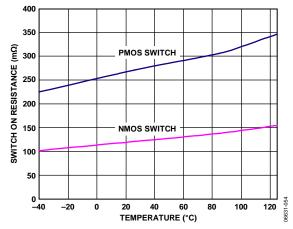
Figure 25. Switch On Resistance vs. Temperature
