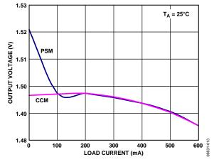
Figure 13. Output Voltage vs. Load Current ( $V_{OUT} = 1.5 V$ )
