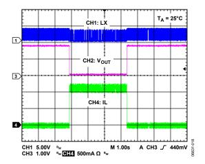
Figure 42. Short-Circuit Response at Output
