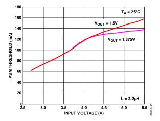
Figure 31. Typical PSM Threshold vs. Input Voltage
