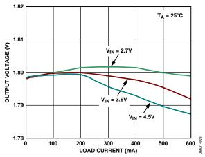
Figure 9. Output Voltage Accuracy ( $V_{OUT} = 1.8 \text{ V}$ )
