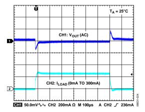
Figure 33. Load Transient Response ( $V_{OUT} = 1.5 V$ )
