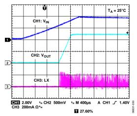
Figure 39. Light Load Start-Up Waveform
