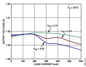
Figure 8. Output Voltage Accuracy ( $V_{OUT} = 1.5 V$ )
