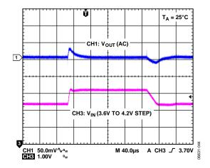
Figure 37. Line Transient Response ( $V_{OUT} = 1.8 V$ )
