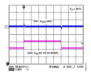
Figure 35. Line Transient Response ( $V_{OUT} = 1.2 \text{ V}$ )
