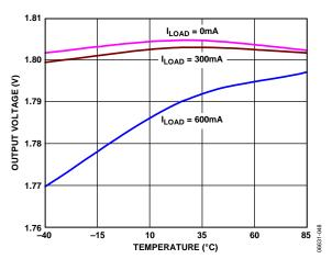
Figure 17. Output Voltage vs. Temperature ( $V_{OUT} = 1.8 \text{ V}$ )
