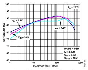
Figure 6. Efficiency vs. Load Current ( $V_{OUT} = 1.8 V$ )
