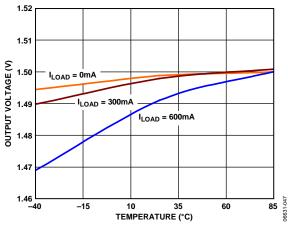
Figure 16. Output Voltage vs. Temperature ( $V_{OUT} = 1.5 V$ )
