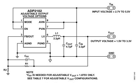
Figure 49. ADP2102 Adjustable Output Voltage Options (0 mA  $\leq$   $I_{LOAD} \leq$  300 mA)
