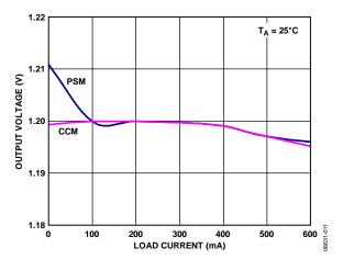
Figure 12. Output Voltage vs. Load Current ( $V_{OUT} = 1.2 \text{ V}$ )
