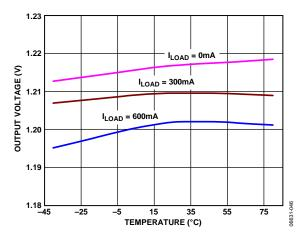
Figure 15. Output Voltage vs. Temperature ( $V_{OUT} = 1.2 \text{ V}$ )
