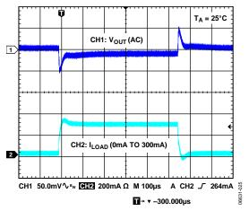
Figure 34. Load Transient Response ( $V_{OUT} = 1.8 \text{ V}$ )
