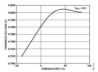
Figure 21. Feedback Voltage vs. Temperature
