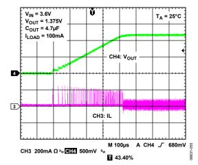
Figure 43. Soft Start Waveform
