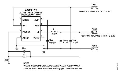
Figure 50. ADP2102 Adjustable Output Voltage Options (0 mA  $\leq$   $I_{LOAD} \leq$  600 mA)
