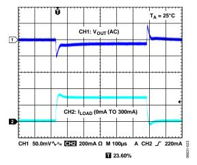
Figure 32. Load Transient Response ( $V_{OUT} = 1.2 V$ )
