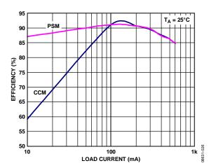
Figure 11. PSM vs. CCM Efficiency ( $V_{OUT} = 1.8 \text{ V}$ )
