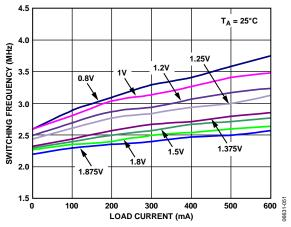
Figure 22. Switching Frequency vs. Load Current
