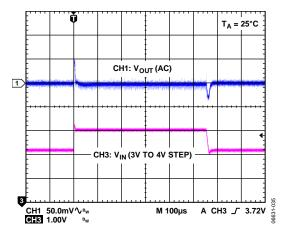
Figure 36. Line Transient Response ( $V_{OUT} = 1.5 V$ )
