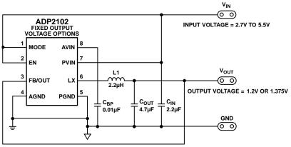
Figure 48. ADP2102 Fixed Output Voltage Options (0 mA  $\leq$   $I_{LOAD} \leq$  600 mA)
