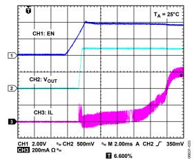
Figure 40. Heavy Load Start-Up Waveform
