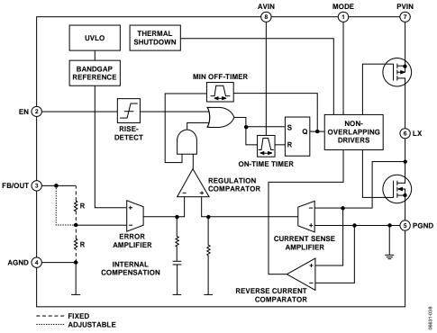
Figure 46. Internal Block Diagram
