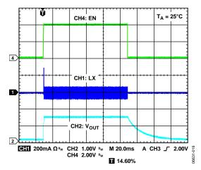
Figure 38. Start-Up and Shutdown Waveform
