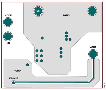
$Figure \, 53. \, Recommended \, Layout \, of \, the \, Bottom \, Layer \, of \, the \, ADP2102 \, Fixed \, Output \, Voltage \, Options \, Application \, Board \, Contract \, Contra$
