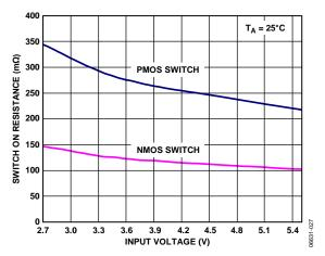
Figure 24. Switch On Resistance vs. Input Voltage
