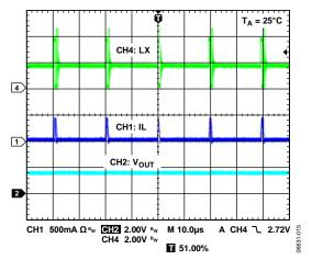
Figure 28. PSM Mode Operation at Light Loads (75 mA)
