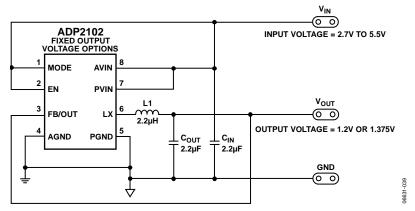
Figure 47. ADP2102 Fixed Output Voltage Options (0 mA  $\leq$   $I_{LOAD} \leq$  300 mA)
