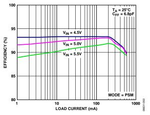
Figure 10. Efficiency vs. Load Current ( $V_{OUT} = 3.3 V$ )
