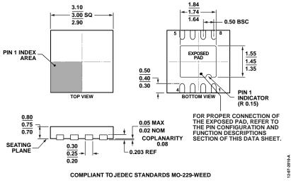
Figure 54. 8-Lead Lead Frame Chip Scale Package [LFCSP] 3 mm × 3 mm Body and 0.75 mm Package Height (CP-8-13) Dimensions shown in millimeters
