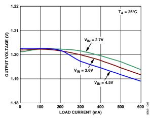
Figure 7. Output Voltage Accuracy ( $V_{OUT} = 1.2 \text{ V}$ )
