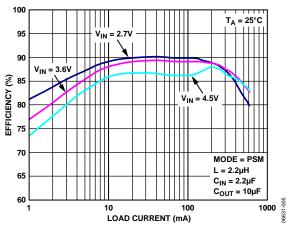
Figure 5. Efficiency vs. Load Current ( $V_{OUT} = 1.5 V$ )
