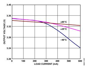
Figure 18. Output Voltage Accuracy ( $V_{OUT} = 3.3 V$ )
