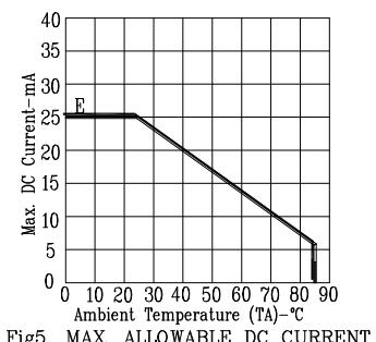
Fig5. MAX. ALLOWABLE DC CURRENT
