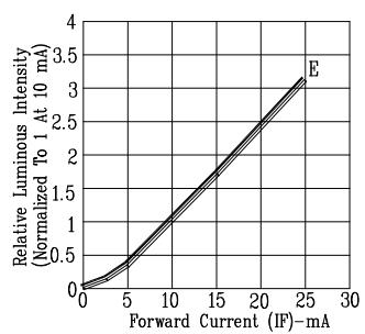
Fig4. RELATIVE LUMINOUS INTENSITY
