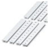
Zack marker strip, Strip, white, labeled, can be labeled with: CMS-P1-PLOTTER, Printed horizontally: Identical numbers 1 or 2, etc. up to 100, Mounting type: Snap into tall marker groove, for terminal block width: 10.2 mm, Lettering field: 10.15 x 10.5 mm
