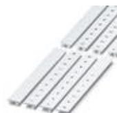
Zack marker strip, can be ordered: Strip, white, labeled according to customer specifications, Mounting type: Snap into tall marker groove, for terminal block width: 10.2 mm, Lettering field: 10.15 x 10.5 mm
