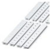
Zack marker strip, Strip, white, labeled, can be labeled with: CMS-P1-PLOTTER, Printed vertically: Consecutive numbers 1 - 10, 11 - 20, etc. up to 991 - 1000, Mounting type: Snap into tall marker groove, for terminal block width: 10.2 mm, Lettering field: 10.15 x 10.5 mm
