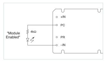
**Figure 4** — LED on-state indicator
