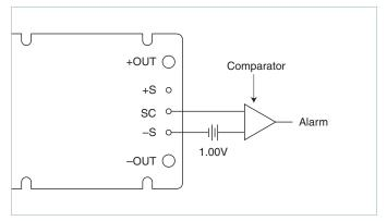
Figure 7 — Secondary side on-state indicator
