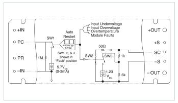
Figure 3 — PC/SC module alarm logic
