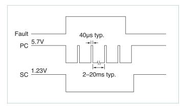
Figure 5 — PC/SC module alarm timing
