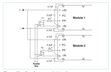
Figure 10 — Transformer-coupled interface
