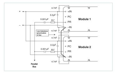
Figure 9 — AC coupled single-wire interface
