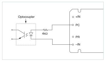
Figure 6 — Isolated on-state indicator
