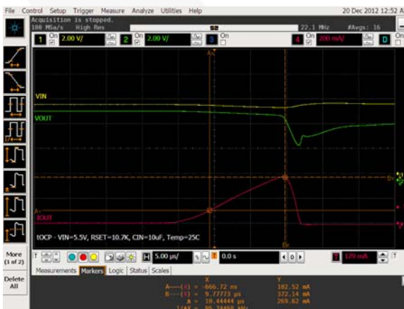
Figure 10. t_{OCP} Response Time
