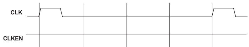
Figure 5-2 Stopping CLK for power saving
