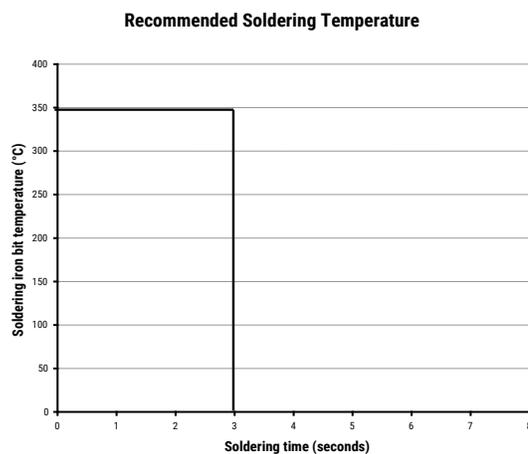
Soldering iron tip temperature should be set at 350°C (+10°C maximum), with the soldering duration not to exceed 3 seconds.
