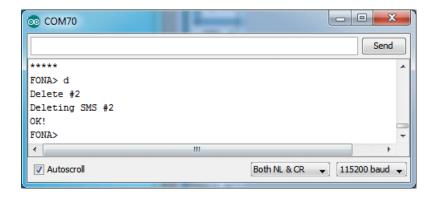
Note that before I deleted SMS #2, so if I read them again, that SMS # will be an empty slot. SMS number #3 doesn't "move slots"!
