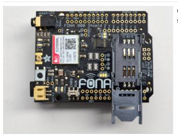
Open by sliding the cover towards the bottom of the shield
