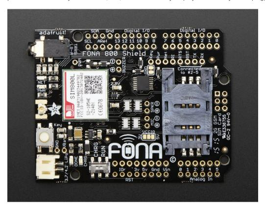
This shield fits on top of any classic Arduino or compatible, and packs a surprising amount of technology into it's little frame. At the heart is a GSM cellular module (we use the latest SIM800) the size of a postage stamp. This module can do just about everything
