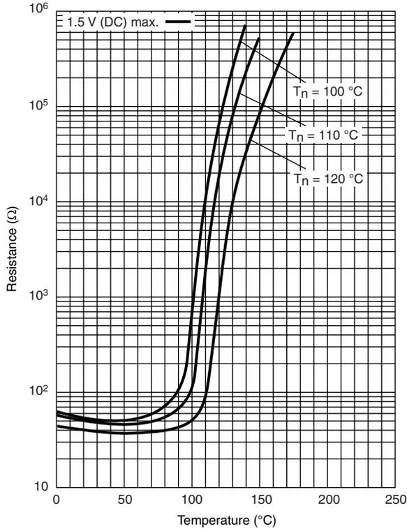
**TYPICAL RESISTANCE/TEMPERATURE CHARACTERISTIC FOR 2381 671 91102/91103 and 91104**
