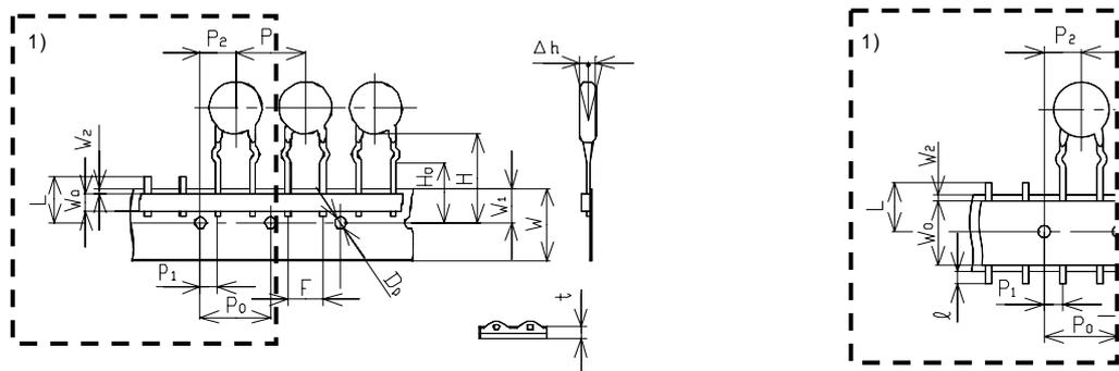
Fig. 1.4 Crimped Leads and Taping
