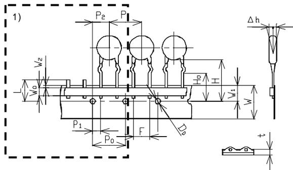
**Fig. 1.4 Crimped Leads and Taping**
