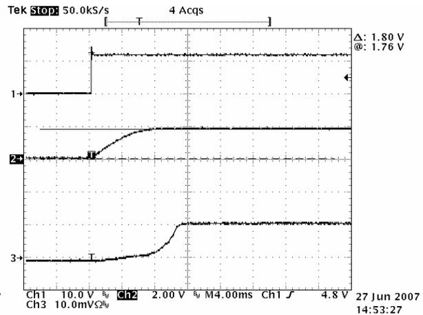
Figure 6- Start up 2A, ch1: Vin
