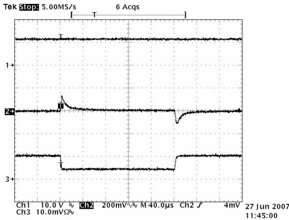
Figure 3- Step load 1-2A, ch1: Vin
