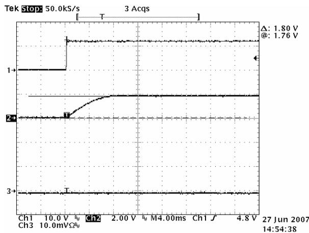
Figure 5- Startup no load, ch1: Vin
