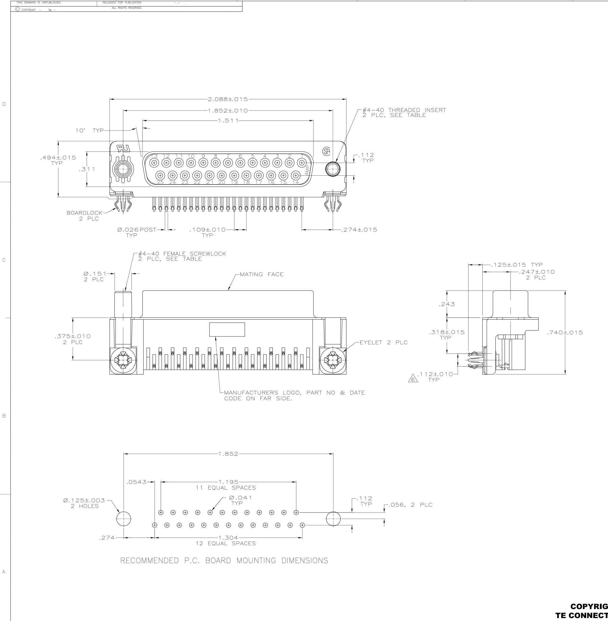
1. CONNECTOR MATES WITH ANY 25 POSN PLUG IN AMPLIMITE SERIES.
