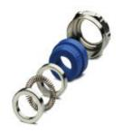
PG21 EMC half screw connection, for size 2 - 4 metal housing, comprising rubber seal, iris spring, cone discs, and pressure screw, for size 1 housing, cable shielding clamping area: 9.5 - 13.5 [mm], cable: 11.5 - 15.5 [mm]
