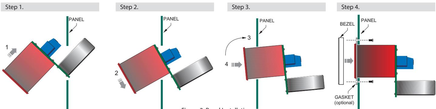
Figure 2. Panel Installation
