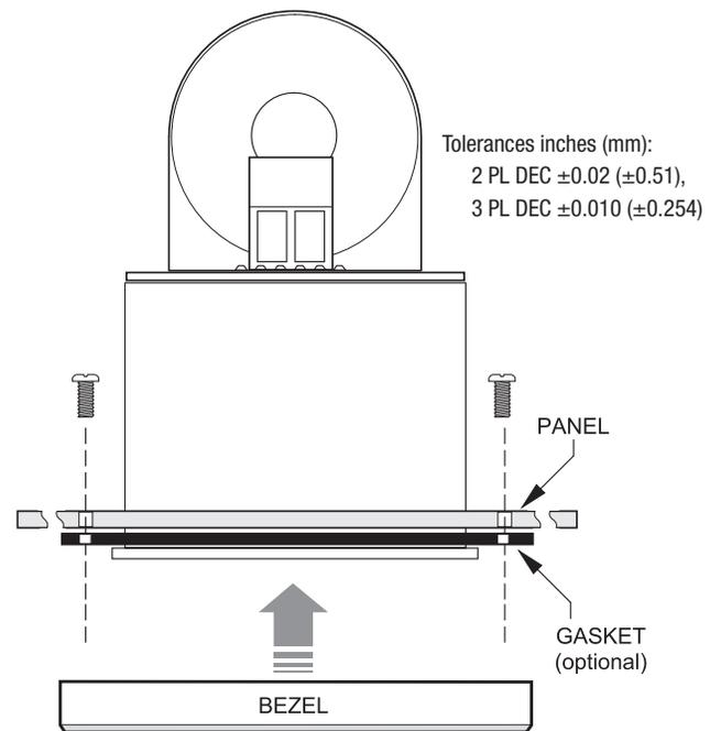
BEZEL INSTALLATION AND RECOMMENDED DRILL AND PANEL CUTOUT DIMENSIONS
