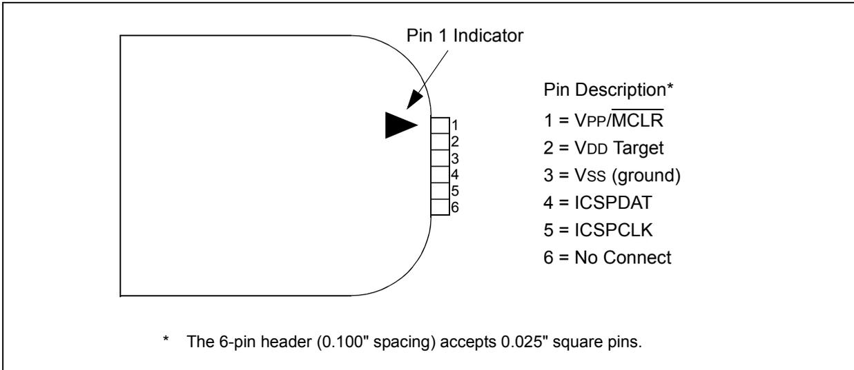
FIGURE 23-3: TYPICAL CONNECTION FOR ICSP™ PROGRAMMING
