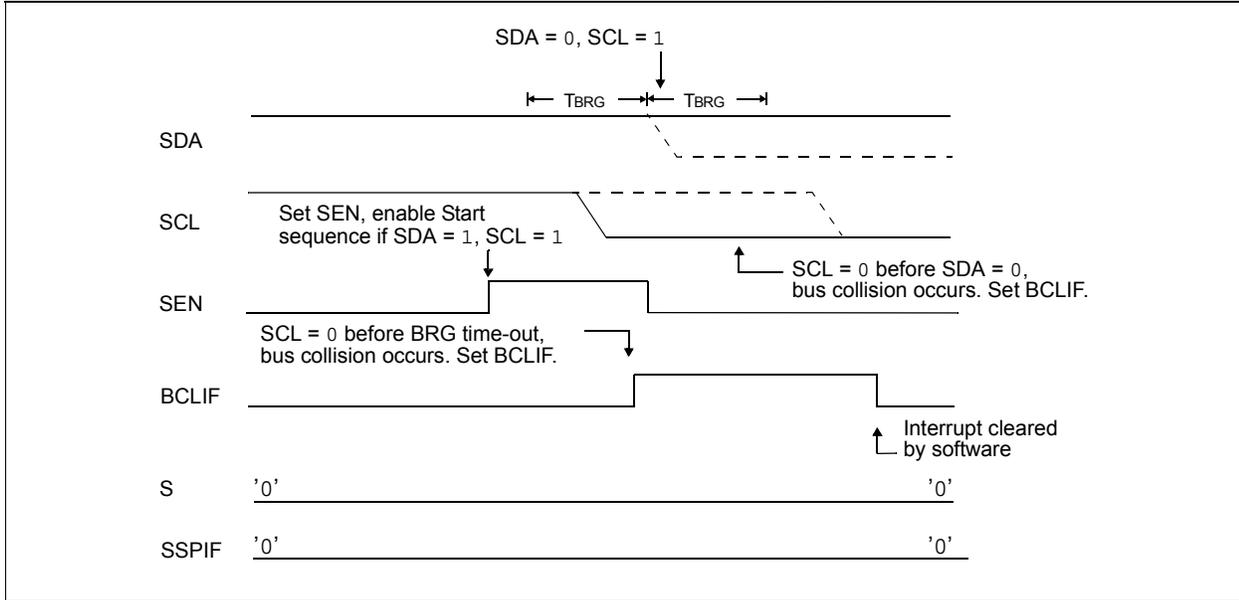
**FIGURE 21-35: BRG RESET DUE TO SDA ARBITRATION DURING START CONDITION**
