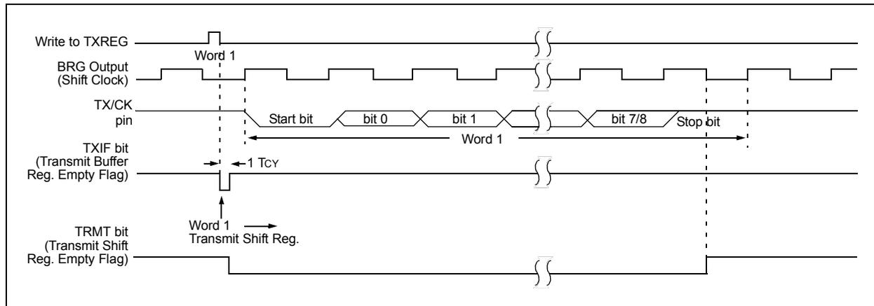
**FIGURE 22-4: ASYNCHRONOUS TRANSMISSION (BACK-TO-BACK)**
