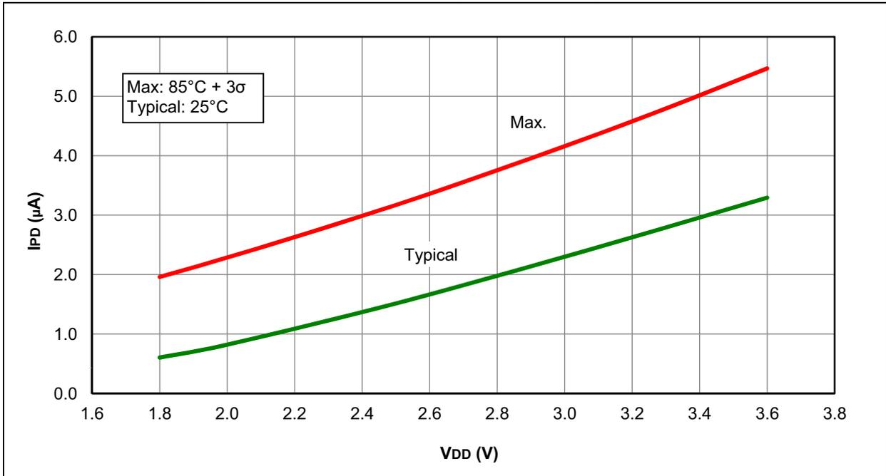
FIGURE 26-40: I<sub>PD</sub>, SECONDARY OSCILLATOR, F<sub>osc</sub> = 32 kHz, PIC16F1516/7/8/9 ONLY
