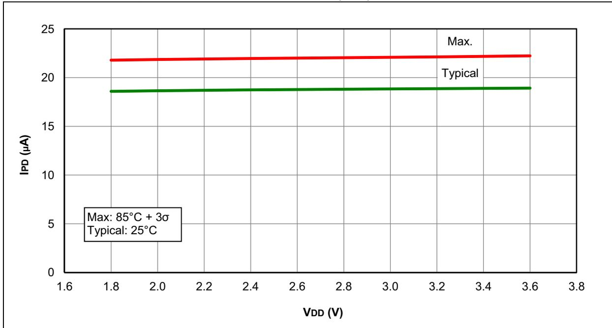
FIGURE 26-36: I<sub>PD</sub>, FIXED VOLTAGE REFERENCE (FVR), PIC16F1516/7/8/9 ONLY
