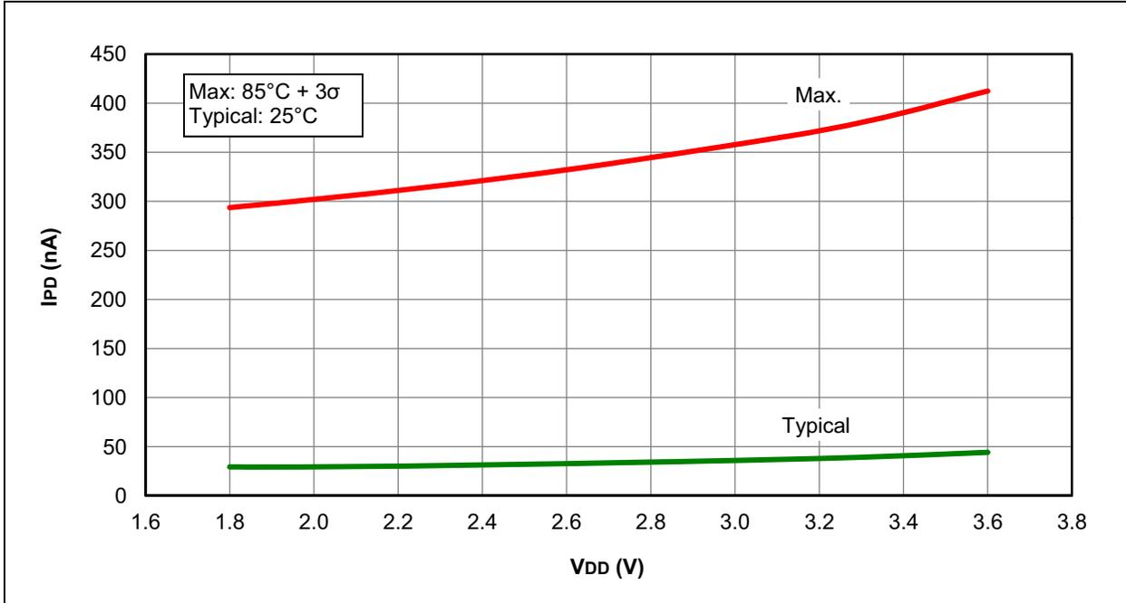
**FIGURE 26-32: I<sub>PD</sub> BASE, LOW-POWER SLEEP MODE (VREGPM = 1), PIC16F1516/7/8/9 ONLY**
