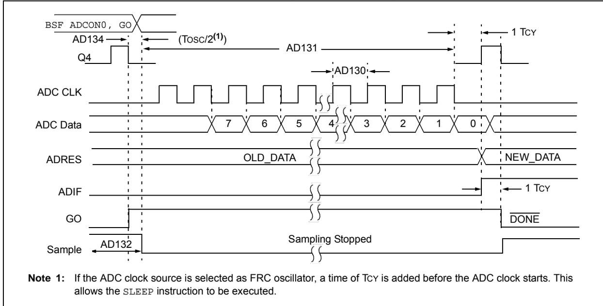
**FIGURE 25-13: ADC CONVERSION TIMING (SLEEP MODE)**
