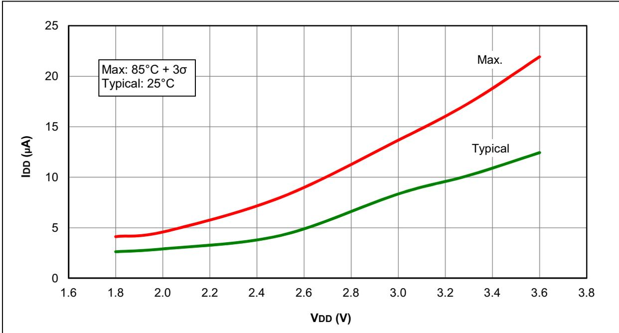
**FIGURE 26-8:** I<sub>DD</sub>, EC OSCILLATOR, LOW-POWER MODE, FOSC = 32 kHz, PIC16F1516/7/8/9 ONLY
