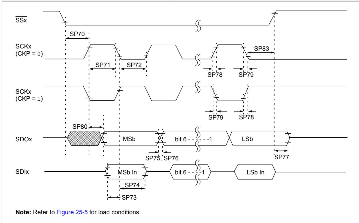
**FIGURE 25-19: SPI SLAVE MODE TIMING (CKE = 1)**
