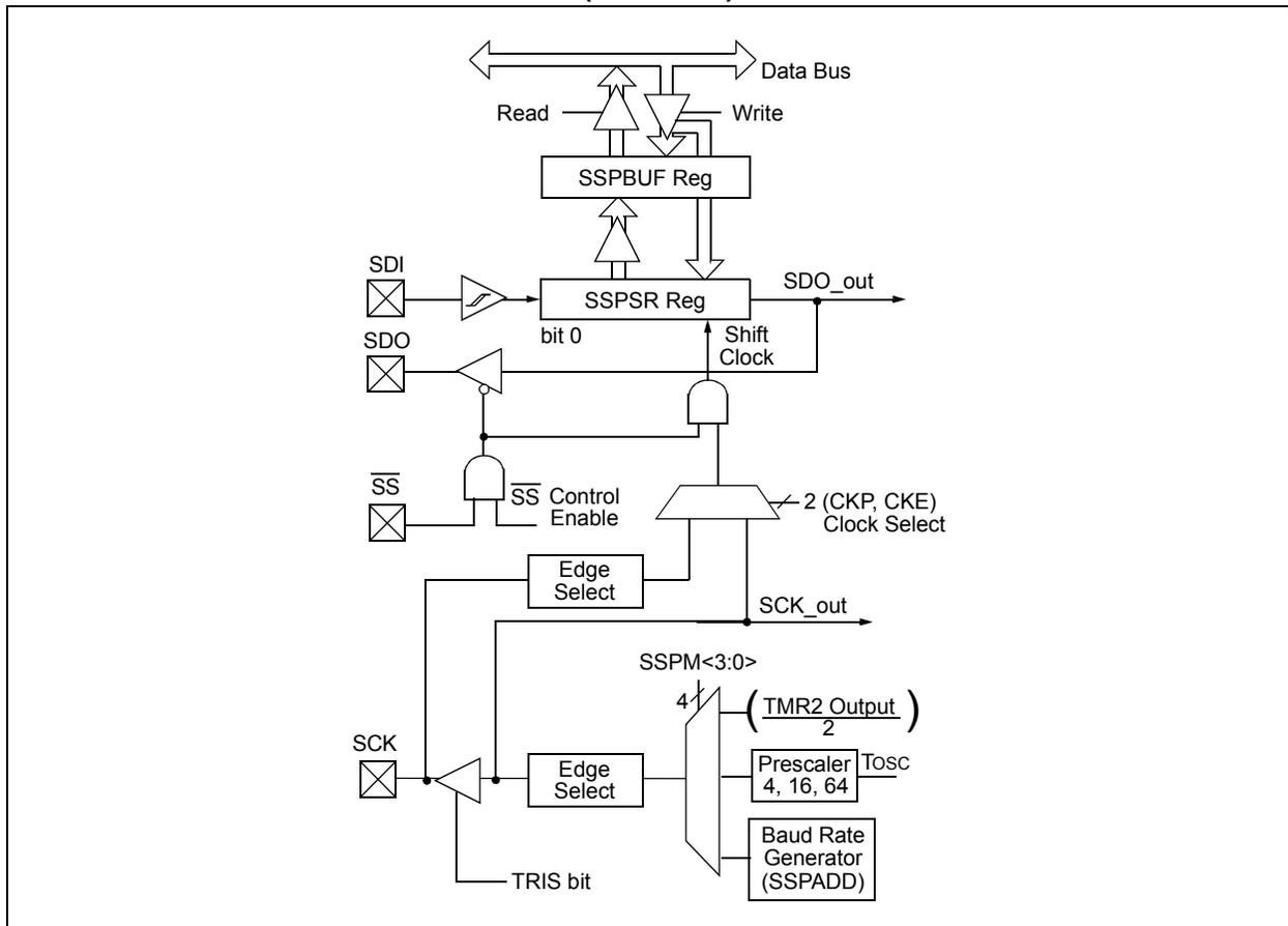
**FIGURE 21-3: MSSP BLOCK DIAGRAM (I<sup>2</sup>C SLAVE MODE)**
