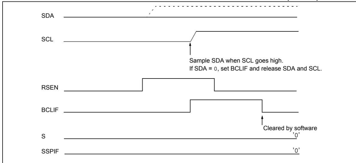
**FIGURE 21-37: BUS COLLISION DURING REPEATED START CONDITION (CASE 2)**
