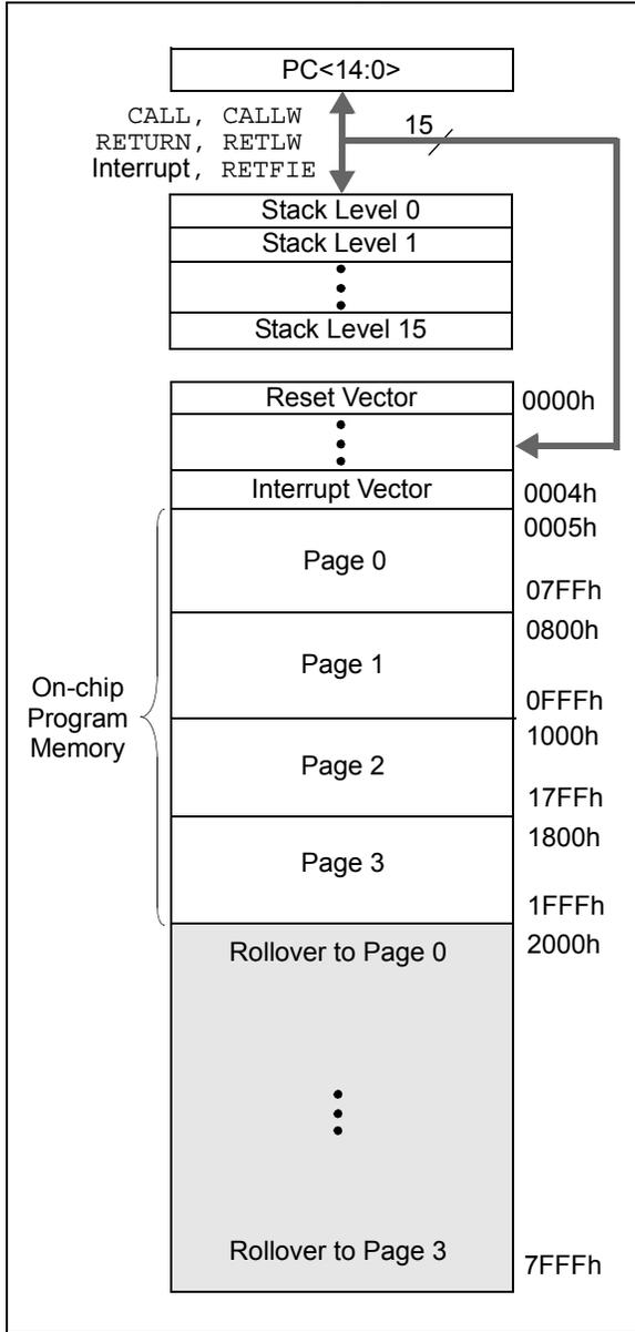
**FIGURE 3-2: PROGRAM MEMORY MAP AND STACK FOR PIC16(L)F1518/9**
