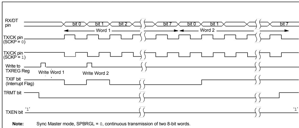
**FIGURE 22-11: SYNCHRONOUS TRANSMISSION (THROUGH TXEN)**
