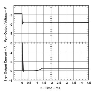
Figure 5. TPS2010, Short-Circuit Current. Short is Applied to Enabled Device,  $V_{I(IN)} = 5.5 \text{ V}$
