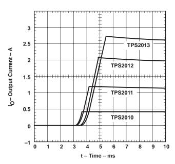
Figure 13. Turned-On (Enabled) Into Short Circuit,  $V_{I(IN)} = 5.5 \text{ V}$
