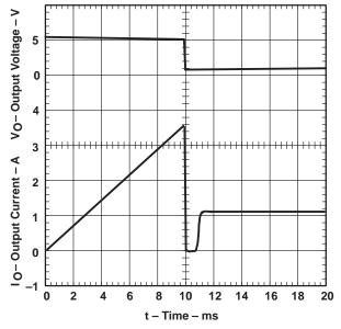
Figure 10. TPS2011 – Threshold Current,  $V_{I(IN)}$  = 5.5 V
