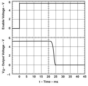
Figure 2. Propagation Delay and Fall Time With 1- $\mu$ F Load, V<sub>I(IN)</sub> = 5.5 V
