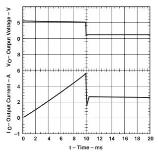
Figure 12. TPS2013 – Threshold Current,  $V_{I(IN)}$  = 5.5 V
