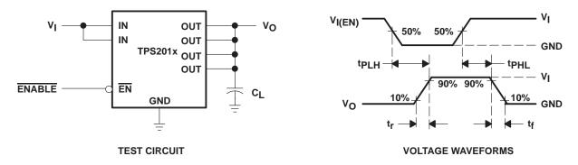
Figure 14. Test Circuit and Voltage Waveforms
