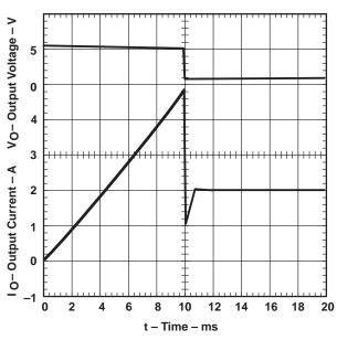
Figure 11. TPS2012 – Threshold Current,  $V_{I(IN)} = 5.5 \text{ V}$
