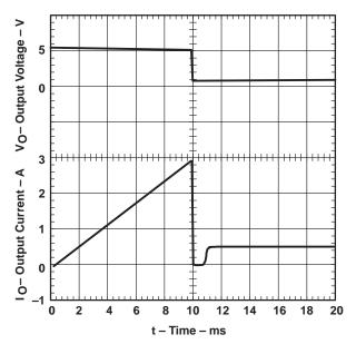
Figure 9. TPS2010 – Threshold Current,  $V_{I(IN)} = 5.5 \text{ V}$
